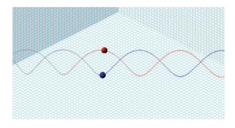
FIG. 6. The two superluminal point-like energy quanta of the superluminal double-helix model of the photon, moving on 45° helical trajectories at a speed  $c\sqrt{2}$ , separated by a distance  $D = \lambda/\pi$  ( $\lambda$  is the wavelength of the photon). Each superluminal quantum composes a spin-1/2 half-photon. Figure from Ref. 34 published under CC-BY license by IOP Publishing Ltd.
