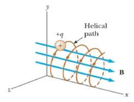
FIG. 1. (Color online) Electron motion in a homogeneous external magnetic field B follows a helical path. Image from Ref. 10, published under CC-BY license by IOP Publishing Ltd.
