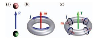
FIG. 5. Electric, Magnetic and Toroidal dipole moments. Image from Ref. 10, published under CC-BY license by IOP Publishing Ltd.
